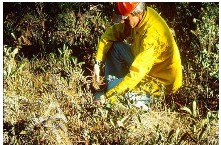
Always check actual on-site conditions as part of your fine fuel moisture estimate by using the snap test or a lumber moisture probe. Photo by Wayne Adkins, USFS Southern Research Station.
