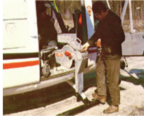
Delayed Aerial Ignition Device (DAID) mounted in a helicopter, Bugwood.org.
